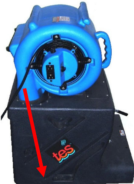
Snout Not Angled Properly
